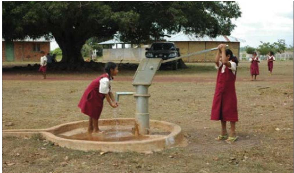
The disadvantages of hand pumps include the exertion required to pump the water and the need to maintain the pumps in good condition which will also need a supply of spare parts. Availability of spare parts is not so much an issue in India where there are many manufacturers of hand pumps. Quality of the water can affect the pump if the water is corrosive in nature. If sand and grit are pumped out along with the water, it can cause wear and tear of the pump too.
